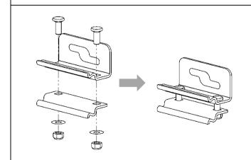
Assemble brackets with a pair of M8 bolts, washers and nuts
